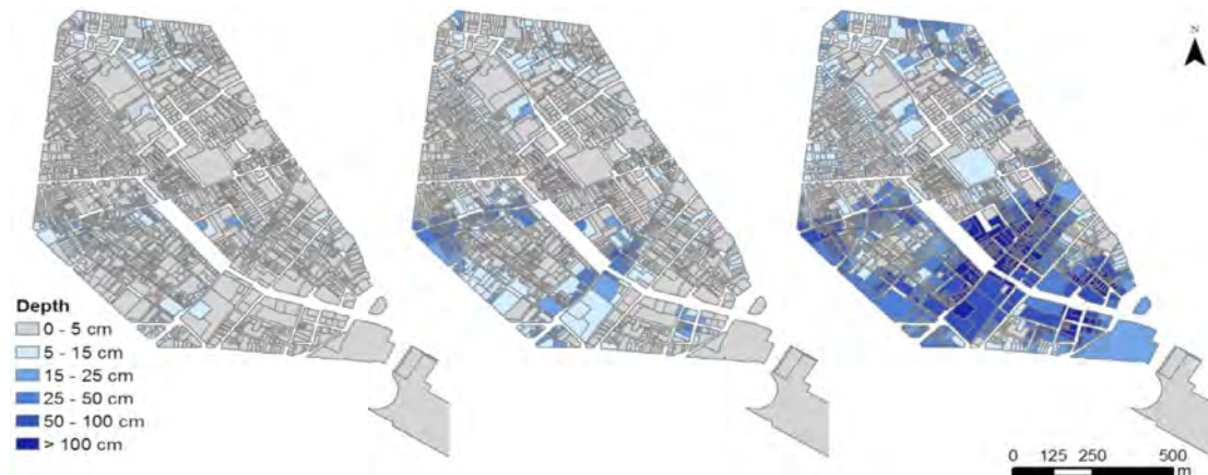
Figure 5 — Flood model results for three different rain events for Raval, with return periods of 1, 10, and 100 years
