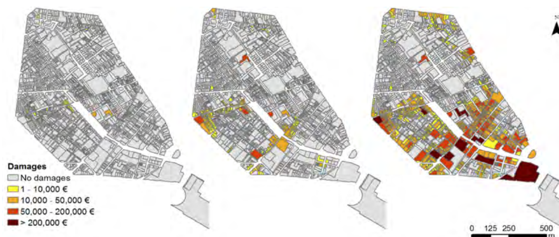
Figure 8 — Flood damages for the three modelled rain events, 1, 10 and 100 years return periods (CORFU, 2014d)
