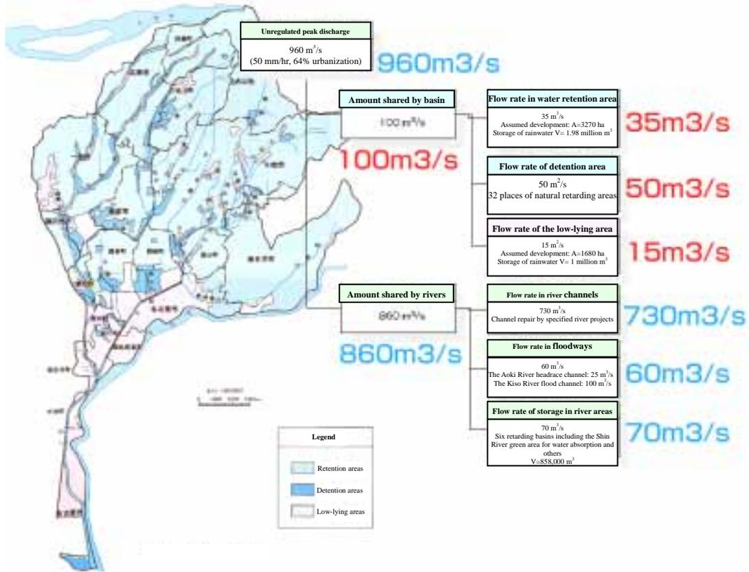
Fig. 31 Basin sharing plan in the Shin River Basin (extracted from the HP of the Shonai River Construction Works Office)
