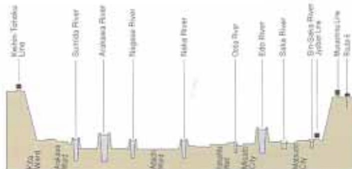
In the city area of London the Thames River flows at the lowest level, whereas in Tokyo the rivers flow at lands located above the city areas, which causes severer damage at the time of a flood.
