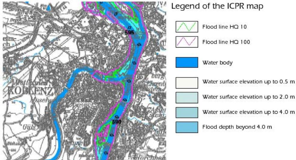
Figure 3. ICPR flood hazard map (ICPR, 2002)
