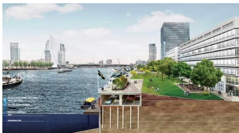
Figure 10 — Dyke enhancement at an urban waterfront in the Netherlands (De Urbanisten)
