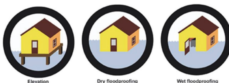
Figure 12 — Different methods of floodproofing (adapted from FEMA, 1986)
