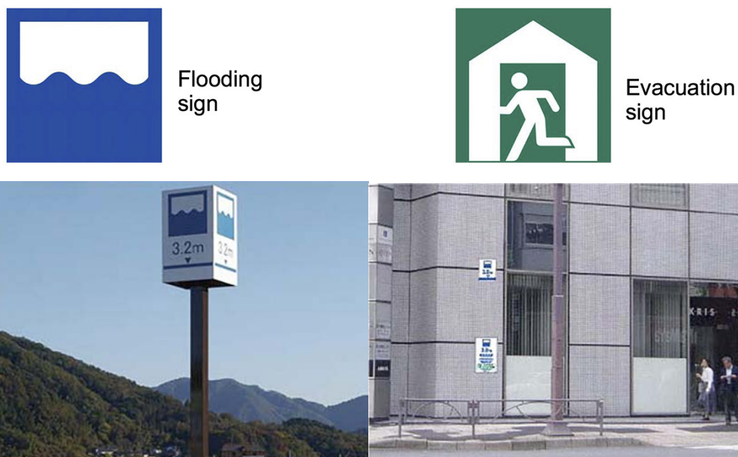
Figure 8 — Standardized marks for flooding in Japan (MLIT, 2006)
