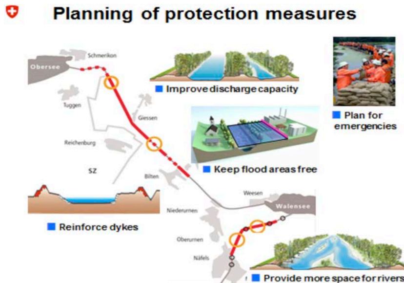
Figure 14 — Specific protection measures
