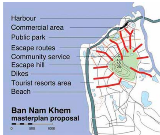
Figure 5 — Map showing a possible protection dike around Ban Nam Khem, in Thailand, with escape routes to safe high areas (CCOP, 2006b)
