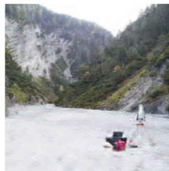
Modern laser scan equipment in use, to determine of the bed load transport movements.
