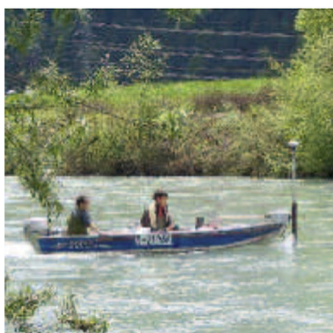
High tech in a measuring boat. Measurement of the Drau river bed with the use of sonar.
