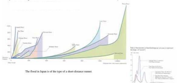
Fig. 5 Comparison of riverbed gradient
