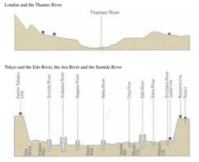
In the city area of London the Thames River flows at the lowest level, whereas in Tokyo the rivers flow at lands located above the city areas, which causes severer damage at the time of a flood.
