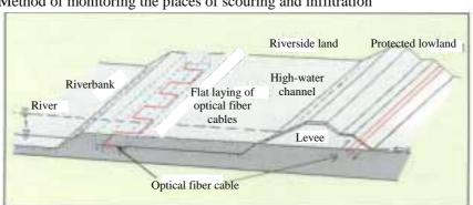
Method of monitoring the places of scouring and infiltration
